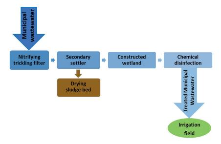
Figure 3. The municipal wastewater treatment process
