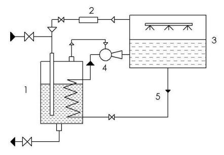
**Figure 1.** Diagram of the installation of periodic physical absorption for an aqueous copper-puddle outlet. 1 – physical desorber, 2 – filter, 3 – pickling machine, 4 – quarterly, 5 – pump.
